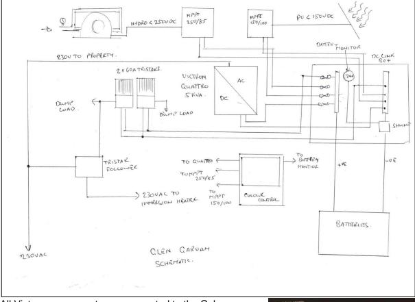
All Victron components are connected to the Colour Control Panel. This gives real time data and also data logging capability. The data can be logged online if the unit is connected to the internet. If no internet is available (as in this case) there is an option to log data to a micro SD card. Note that the output hydro output is 602W. This is 18% higher than predicted by the calculator. This outcome is normal for well installed PLT turbines.
